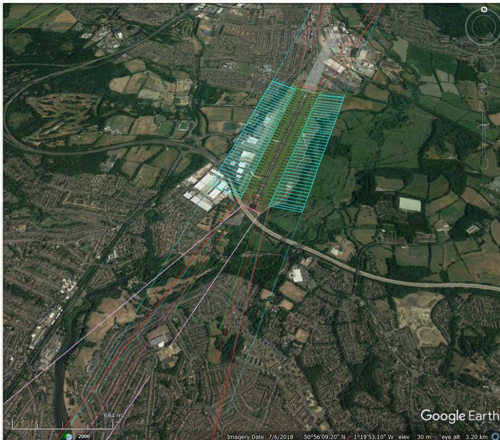
Example of the Obstacle Limitation Surfaces at Southampton Airport overlaid on Google Earth
